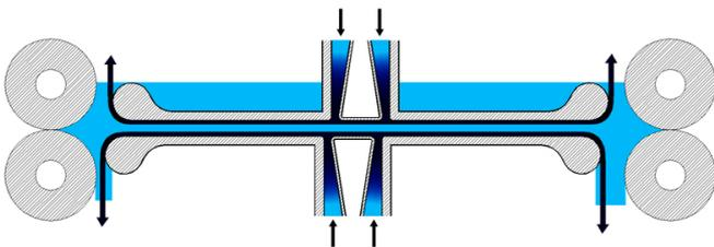
at the centre of each plate via continuous slots or knives, resulting in steady boundary layers balancing and guiding material in transit. The leading
