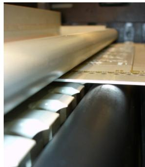
and trailing edges of the plates are shaped to take advantage of Coander effect, diverting the boundary layer diffusion point away from the panel entry and exit zones. This maintains the streamline flow and diverts fluid above the plates, preventing flooding and material deflection.
