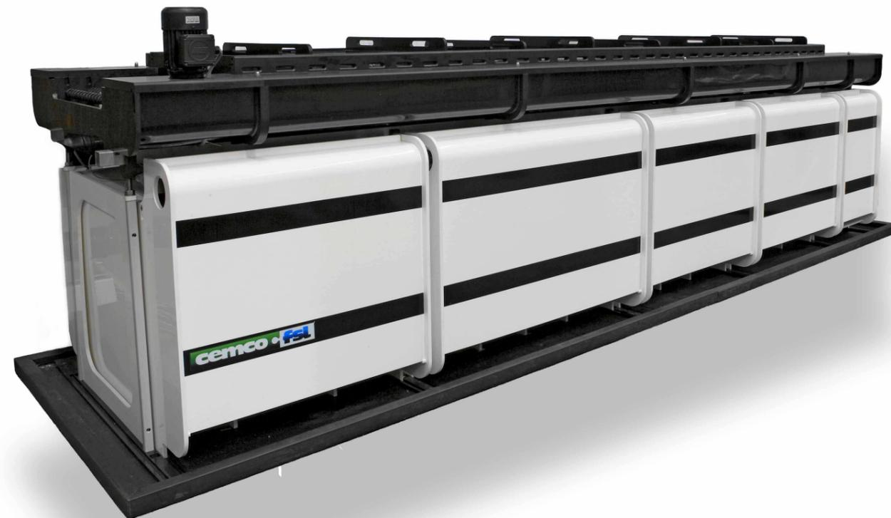
This new product range takes its name from the unique laminar or streamline flow treatment chambers that replace conventional flood and spray chambers used in earlier designs. These fluid engines result in faster and more uniform reaction, reducing processing time and equipment footprint. This is only one of the unique features that make the **Streamline** range smaller, more efficient and more capable than conventional equipment....
