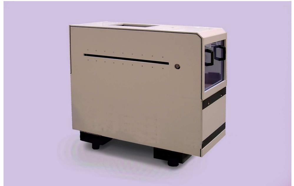
The airknives are quickly detachable for ease of cleaning. The Dryer is made of PVC shell construction. It incorporates an energy efficient side-channel compressor complete with variable speed control to enable performance to be matched precisely to application. There are no internal heaters and therefore reduced operating costs. The air knives are machined from billet aluminium to guarantee product stability, and are coated with a durable hard-anodised finish for long life.
