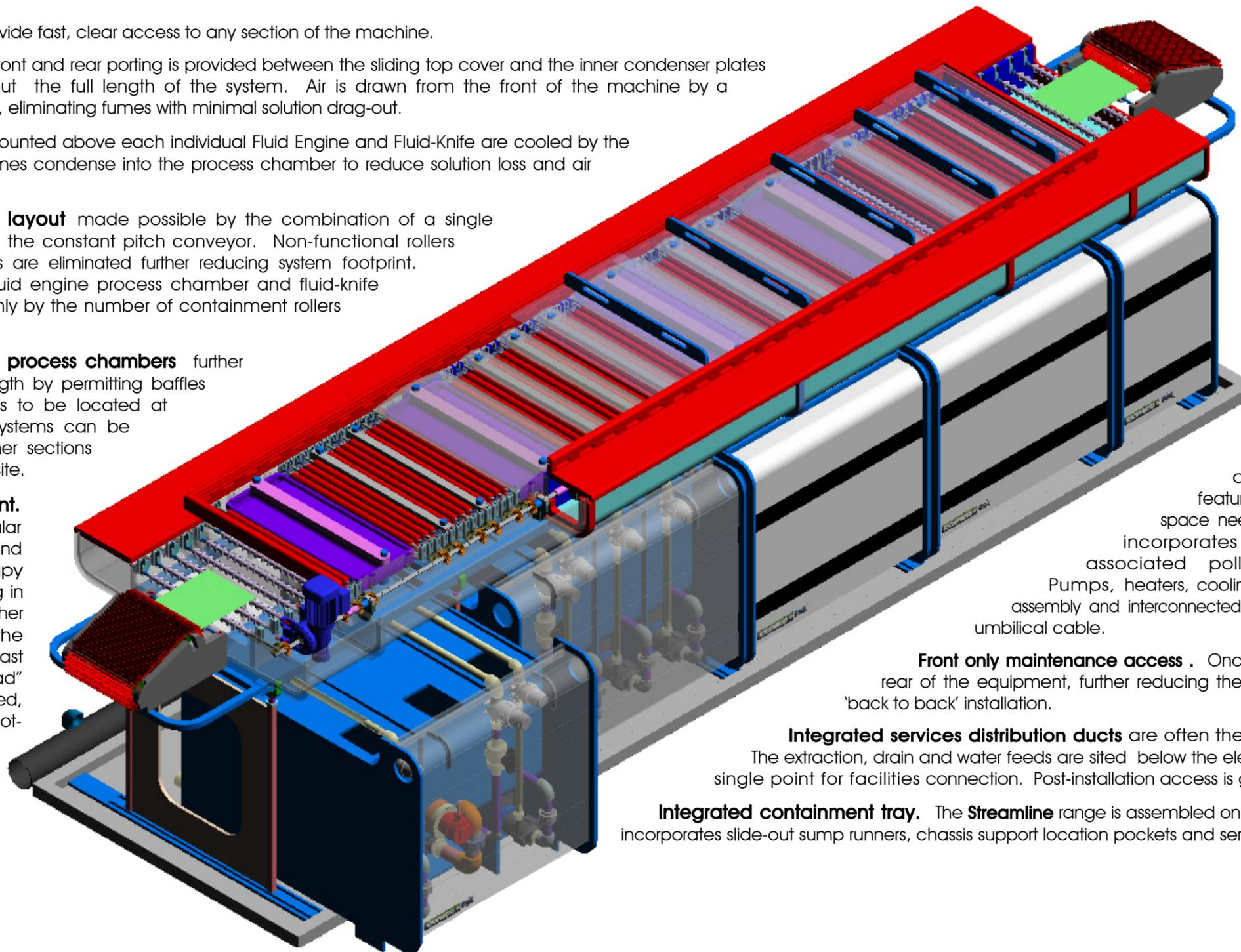
**De-coupling chassis.** The upper conveyor/process chamber assembly is supported and located on chassis rails that permit movement in the long axis. By decoupling the process chamber and sump, warp, twist and yaw resulting from heating and cooling is eliminated. **Streamline** board handling equipment can be plugged into the chassis rails and support legs provide leveling adjustment at the top of the leg away from spills.
