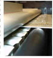
and trailing edges of the plates are shaped to take advantage of Coander effect, diverting the boundary layer diffusion point away from the panel entry and exit zones. This maintains the streamline flow and diverts fluid above the plates, preventing flooding and material deflection.
