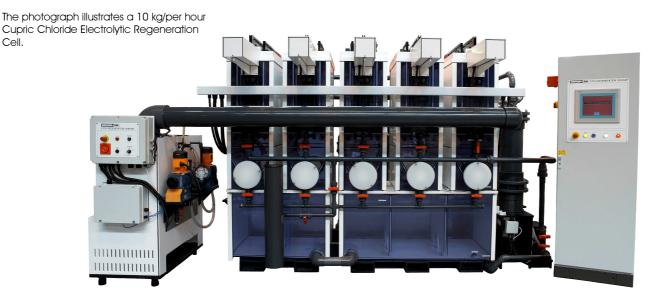
CEMCO manufacture Regen systems in a range of sizes. They are built as 2kg (4.4 lb)/per hour cell modules. This refers to the recovery rate of copper per hour. Modules can grow in size to a maximum of 10kg (22 lb)/per hour. Thereafter multiples of modules can be used in series with one another to suit any size production.
